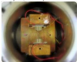
An internal view of the vacuum chamber containing the fusion device, showing two pyroelectric crystals that generate a powerful electric field when heated or cooled. Photo by Rensselaer/Yaron Danon
