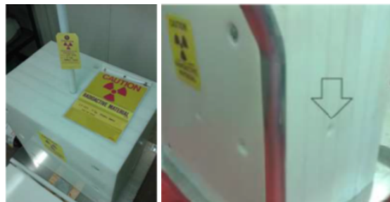
Fig. 4. (Left) The polyethylene cube with a ^{252}\text{Cf} spontaneous fission source in the center used for neutron flux measurements (Right) The experimental port used for the solid state neutron detector used to measure the flux in the cube as a function of the position.
