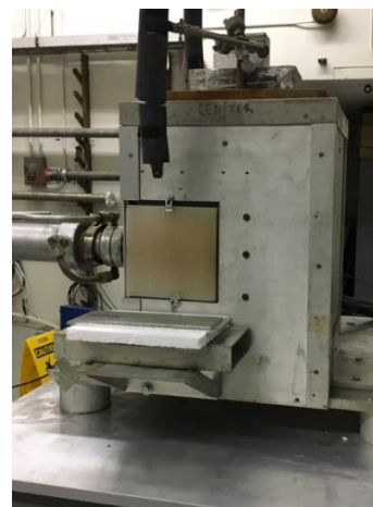
Fig. 1: ETT side view where neutrons leave in the direction of detectors.
