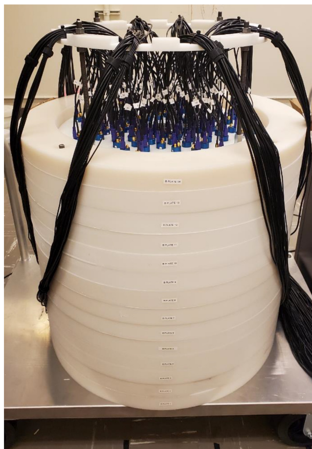
Fig. 4. Photograph of the as-built detector system. The system was constructed on a cart with wheels for ease of maneuverability and can pass through doors wider than 81.28 cm (32 in.).
