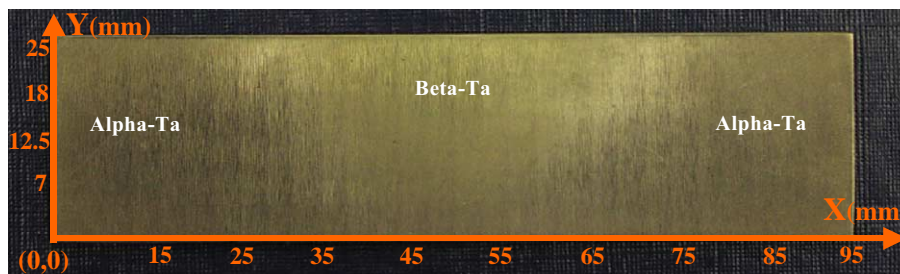
Fig. 6. Surface image illustrating the distribution of alpha (darker phase) and beta (lighter phase) tantalum across the surface of the sample.
